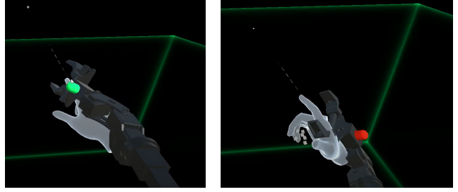
Figure 6. (left) The green light shows that the user input is a feasible pose for the robot. (right) The red light shows that the robot is not able to reach the pose provided by the user.
