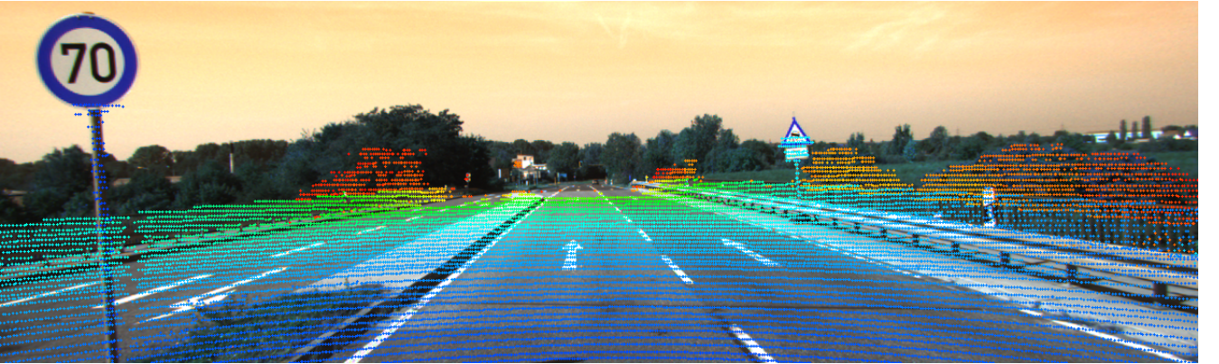
Figure 11: Point cloud projection on image '0000000037' after motion distortion has been corrected
